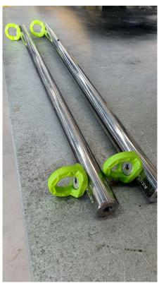
Lifting Gear Hire & Sales can provide a full rigging set-up including small modular spreader beams that can be assembled in 100mm increments plus round slings and any other rigging.
